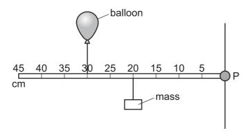
The balloon is filled with helium, a gas less dense than air, so that it applies an upward force on the rod.
